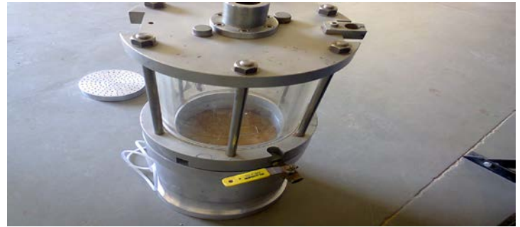
Fig. 3. Modular-leaching column device
